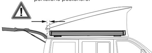
**EN** **ATTENTION** Periodically check the brackets to make sure they are firmly attached (especially after the first kilometers) make sure the bolts are not loose and that holding brackets have not shifted.
