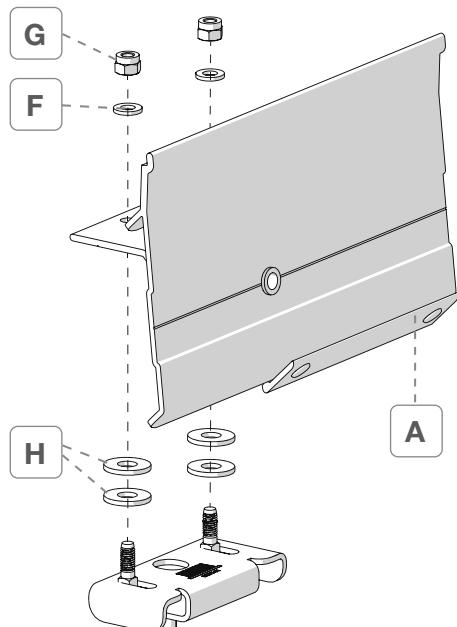
**EN** The "H" washers should only be used, where necessary, to compensate for an excessive gap between the roof of the vehicle and bracket.
