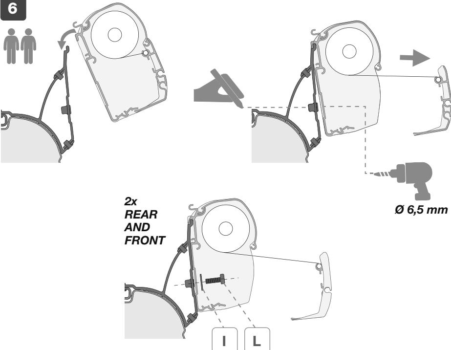
**EN** Before tightening the screws, make sure that the awning position doesn't prevent the opening of the rear door.
