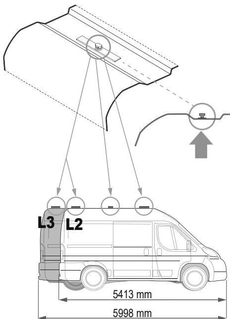
**EN** **Attention:** to fix the brackets, use exclusively the hookings that are on the vehicle.
